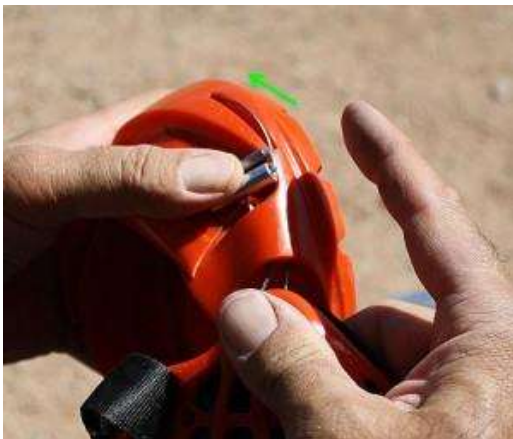
14. Considering that you still have one cable remaining, go to that side of the boot and push the end of the cable through to the other side until the end pokes out like shown below. You might not get this much cable to come out but if you can see the end of the cable that is good enough.
