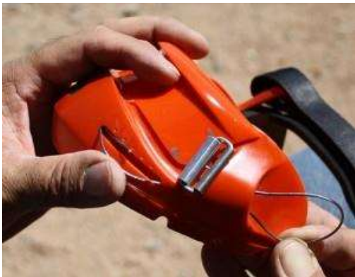
17. Push the new cable on through until you can also see the end poke out on its opposing side as shown below.
