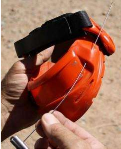
12. Install a new cable into the top Guide-Way hole first.
