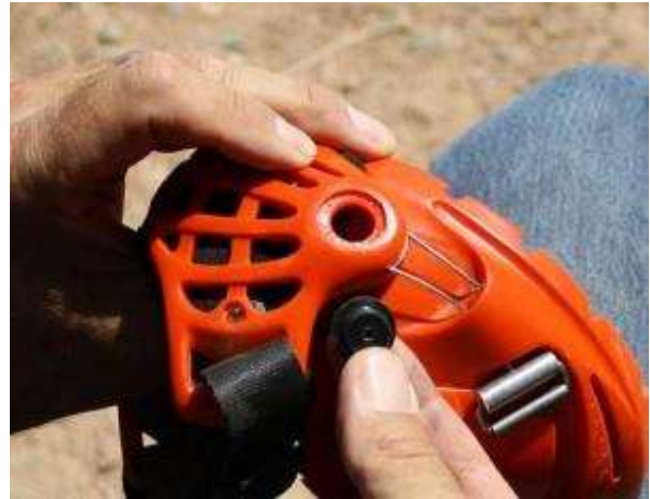
22. Be sure the cable loop is all the way back into the slot, which clears the hole. Reinsert the big half of the pulley button from the inside.
