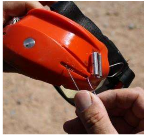
16. It's easy now to insert the new cable without the cable ends butting heads inside the tunnel.
