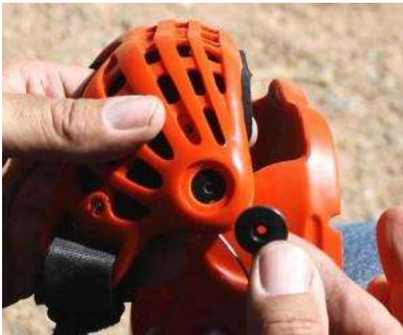
23. Insert the small half of the pulley button from the outside.
