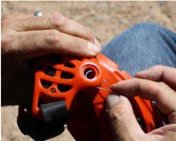
21. Now insert the cable loop into the slot on the end of the heel captivator.
