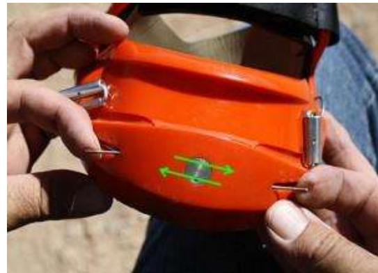
18. The arrows depict what the cables are doing inside the clamp.
