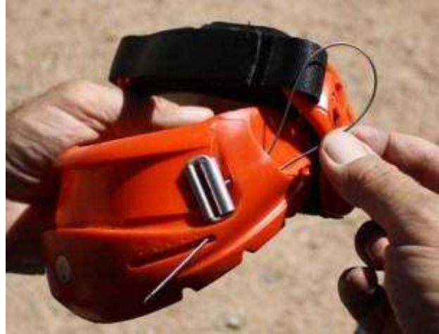
13. Now insert the cable through the lower Guide-Way hole so that it forms a loop like this.
